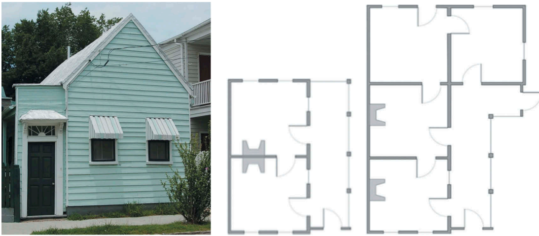
Figure 5. Traditional freedman's cottage in Charleston (left); examples of traditional freedman's cottage floor plans (center and right) (source: Felzer 2008).
